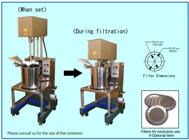
At screen printing, there are occasional problems such as open-circuit, short, and void due to impurities in the pastes.PF series are cutting-edge products to eliminate such impurities efficiently and automatically.
